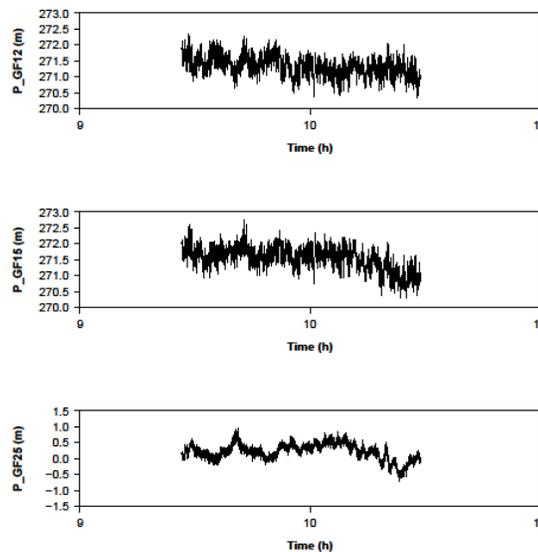
**Figure 34: Geometric-Free code combination for station GMIZ Day of Year 341 in 2008 – Both L1/L2 and L1/L5 combinations vary around 270 m, whereas L2/L5 vary around 0 m. We found out that it could be explained if L2 and L5 code hardware delays are rather small, while L1 ones rather large.**
