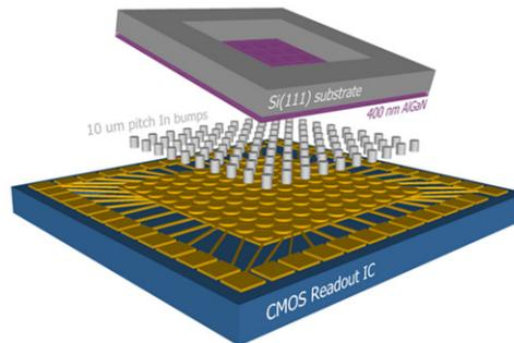
Figure 52: BOLD prototype design
