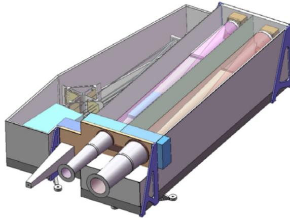
**Figure 59: 3D view of the EUI optical bench (CEB not shown)**
