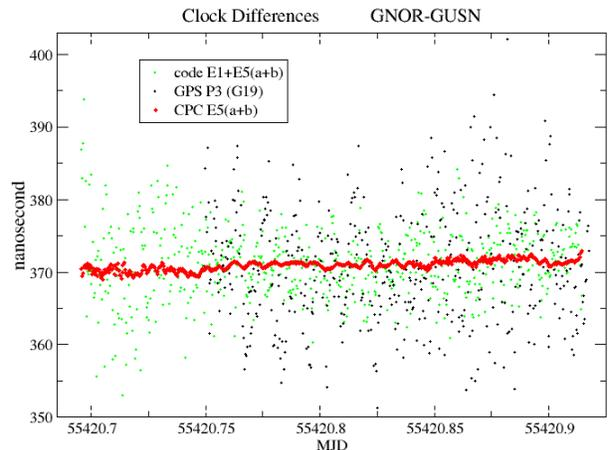
**Figure 11: Comparison between the clock solutions obtained with either dual-frequency ionosphere-free combination of pseudoranges, or the CPC combination.**
