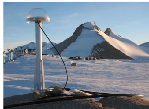
**Figure 15: GPS antenna installed at the Princess Elisabeth base in Antarctica**
