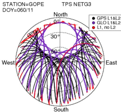
**Figure 14: Snapshot of the tracking for the station GOPE showing the skyplot for a particular day.**
