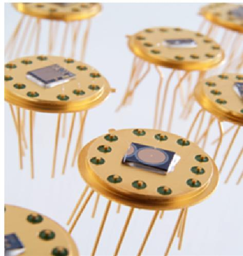
Figure 53: Single UV photodiodes (IMEC)
