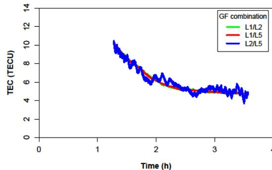
**Figure 35: TEC values for station GNOR Day of Year 013 in 2008:  $TEC_{25}$  is less precise than  $TEC_{12}$  and  $TEC_{15}$ .**
