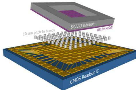
Figure 52: BOLD prototype design
