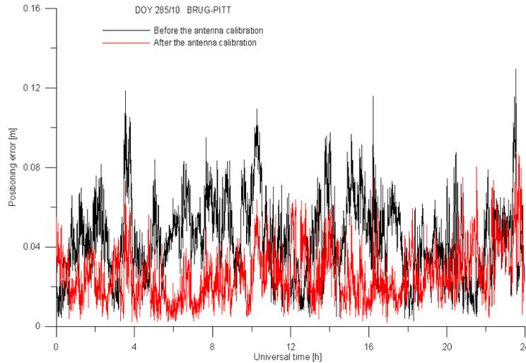
**Figure 36: Positioning error given by SoDIPE software for the baseline Bruges (BRUG) – Pittem (PITT) before (black line) and after (red line) the antenna calibration for DOY 285/10**
