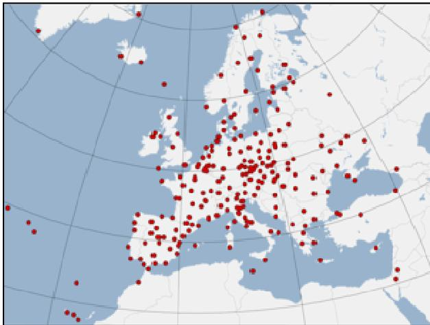
Figure 12: Map of the continuously observing GNSS stations in the EPN (Status: March 2010)
