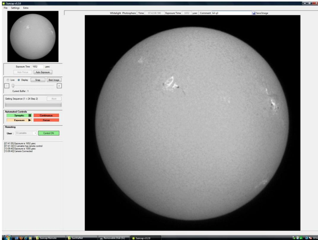
**Figure 47: Screenshot of the new streamlined SunCap graphical user interface. The new program features improved and extended capabilities for automated image acquisition and is ready-built for future extensions (remote control of pointing and focus, etc.).**
